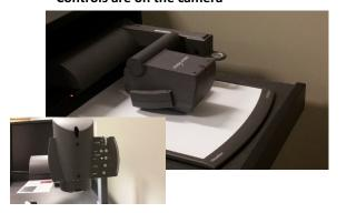
Controls are on the camera; Push the button in back to release lamp arms and camera
