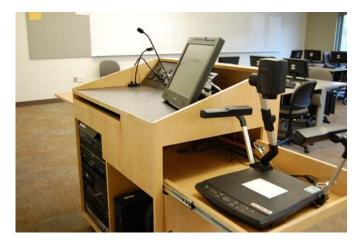
Once the slider is pulled out, you can click the camera head into place and adjust the lights to your need. After you have turned on the podium power and selected "Doc Cam" from the display device options across the top, depress the green power button on the document camera to turn the power on. Whatever is placed on the document stand will be displayed on the projector and the desktop monitor. You have camera like controls available for zoom, focus, iris, etc. as in the picture below.
