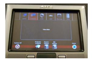
From this screen, simply select the device you wish to display from the options across the top of the touch screen. The system will turn on and your display device will be selected.
