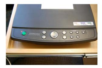
Please note there is a rotate button on this unit that rotates the image in increments of 90 degrees so you can orient your materials however you need.
