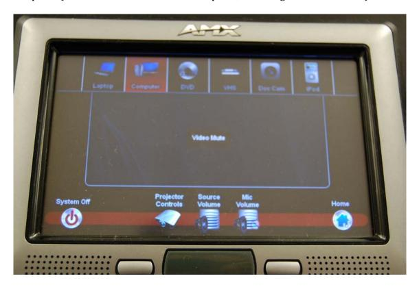
At the bottom left corner of the AMX touch screen control, there is a button labeled "System Off". Upon touching this button, you will be prompted to confirm you wish to shut down. Confirm this message by touching confirm and the system will shut down. This includes projector off, screen retract, and video to local desktop monitor turns off. Please note that the devices mounted in the podium will still have power. You do not need to turn off anything else at this point.
